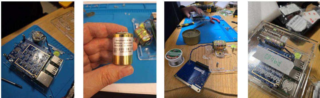
Figure 4. Replacement of vertical geophones by horizontal geophones of the RS4D accelerographs.
