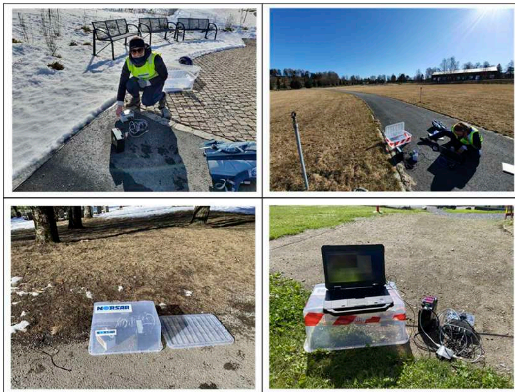
FIGURE 2 Pictures taken during fieldwork in the Alna and Blindern regions (1 and 3 area in Figure 1) in March and June 2021. On the top left, deploying the instruments at the site. On the top right, writing down the starting time of the recording and coordinates information related to the site. In the bottom left, the instrumentation is recording at the site for 1 hour. In the bottom right, downloading the recordings on the laptop.
