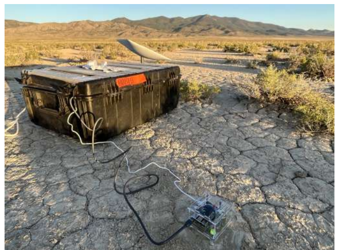
Figure 2 Instrument setup. The PiShake is visible as the transparent box in the foreground, with the geophone and infrasound sensor mounted within the same instrument and levelled using the built-in spirit level. Power (white cable) and data (black cable) are routed through the weatherproof black box. The generator and acoustic baffles are not shown, but the Starlink connection is visible in the background. The unconsolidated alluvial surface and range of hills with peaks 5-10 km away are also visible. Image direction: north (toward EDL trajectory).
