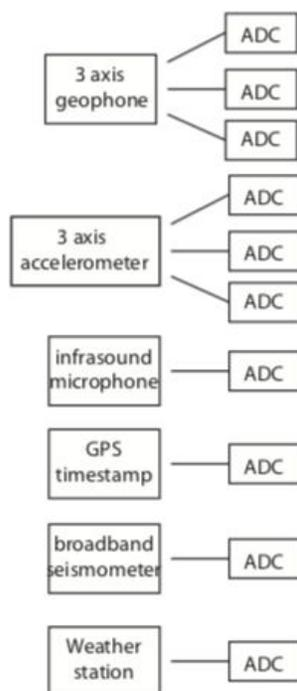
Figure 2: Overview of potential components and data transfer specifications. ADC are 24 bit and proposed sampling rate is 100 Hz.
