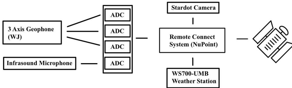
Figure 1: Approximation of componentry of the MMVC monitoring project.
