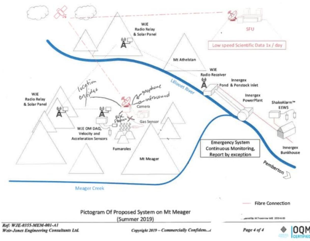
Figure 6: System Pictogram from WJE, with markups by QUC. QUC system is in red.
