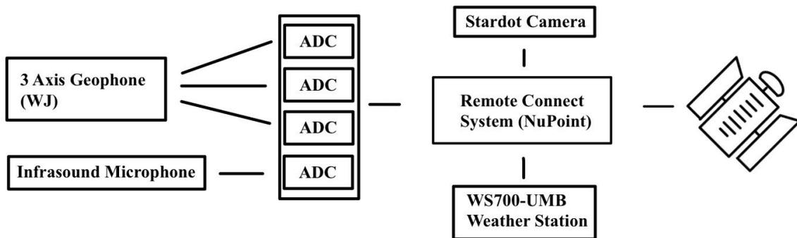
Figure 1: Proposed componentry for the QUC-MMVC landslide monitoring system
