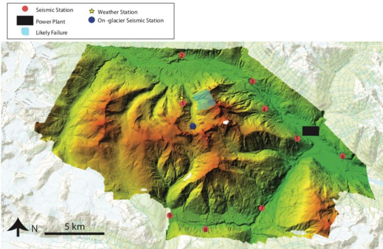
Figure 1: LiDAR Map of the MMVC Monitoring Network. Preliminary Locations of seismic stations were chosen based on known bedrock (Read et al., 1978) and preliminary line of sight analysis.
