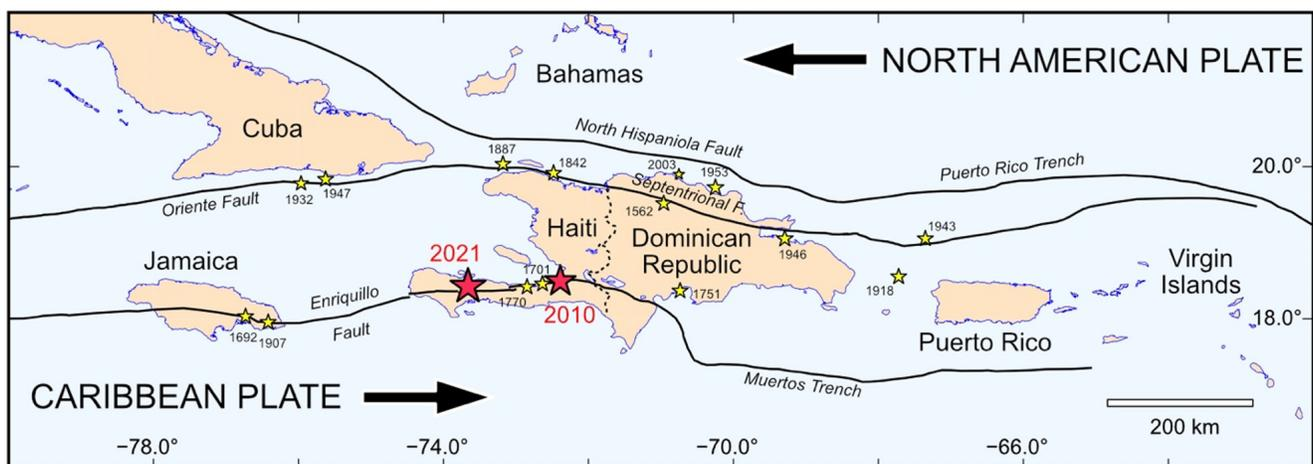
**Figure 1** Location map. Haiti and the Dominican Republic share the island of Hispaniola. The black lines indicate the major seismic faults, which accommodate the movement between the North American (north) and Caribbean (south) plates whose relative displacement (2 cm/year) is shown by the black arrows. The most important historical earthquakes in terms of damage are indicated by yellow stars. The red stars indicate the epicenters of the earthquakes of January 12, 2010 and August 14, 2021.
