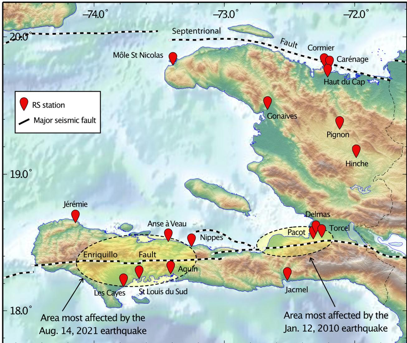
**Figure 3** Map of the location of Raspberry Shake stations in Haiti at the time of the interviews (red) and subsequently installed (yellow), as of October 24, 2021. Regions affected by the 2010 and 2021 earthquakes are indicated approximately by yellow ellipses.
